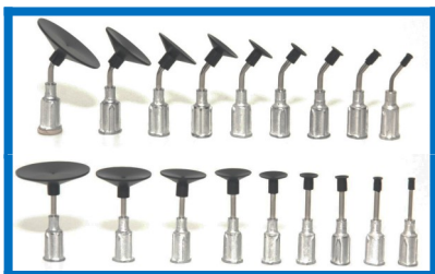
ESD safe vacuum tips available in Buna-n or high temperature silicone rubber. Sizes range from 3/32" (2.38mm) to 1" (25.4mm).
