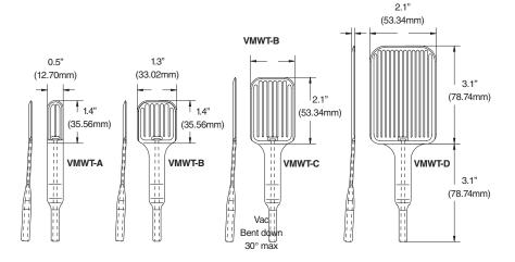
Molded Wafer Tips VMWT-A, VMWT-B and VMWT-C are available with a 10°, 20° or 30° bend in the up or down direction as shown in the left drawing above. To order a tip with the up or down bend, add the angle plus a "U" for up or a "D" for down to the part number. EXAMPLE: Part number VMWT-A20D is a VMWT-A Wafer Tip with a 20 degree bend in the down direction. Custom angles are available upon request. Pricing is as above.
